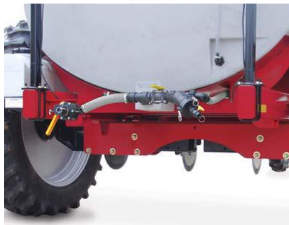
The plumbing and wheel adjustments are conveniently located for easy access.
