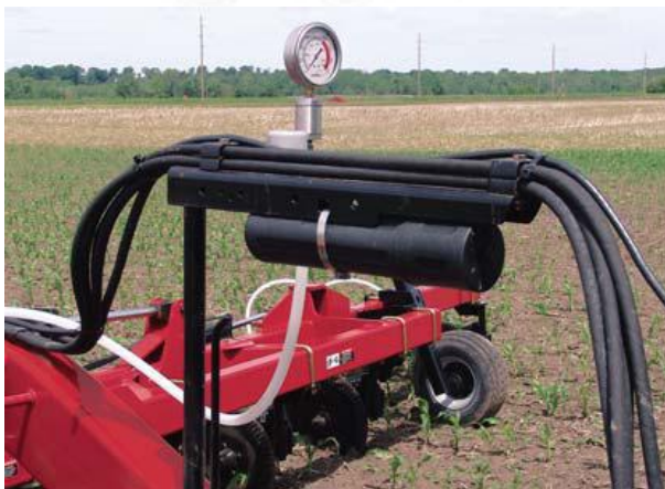
The front hose stand keeps hoses and wires away from the tractor hitch.
