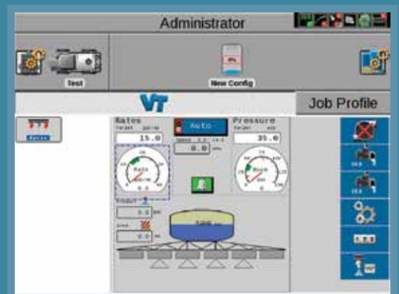
The Hawkeye System is built on the ISOBUS communication platform which allows it to work with ISO Task Controllers, including the Viper® 4.
