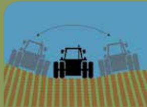
SmarTrax offers 3D terrain compensation for maximum accuracy and repeatability, automatically adjusting for tractor roll, pitch and yaw.
