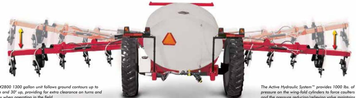
The NPX2800 1300 gallon unit follows ground contours up to 6° down and 30° up, providing for extra clearance on turns and flexibility when operating in the field.
